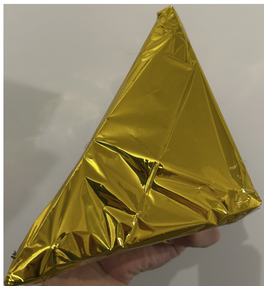
Figure 2 - Mylar covering for NOVA payload
